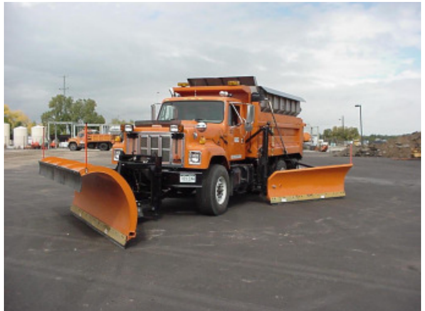
A tandem plow with a V-box for applying solid de-icers and a plow on the front and side to increase plowing activities without increasing manpower or equipment needs. CDOT has eight tandems with wings in the Denver metro area.
