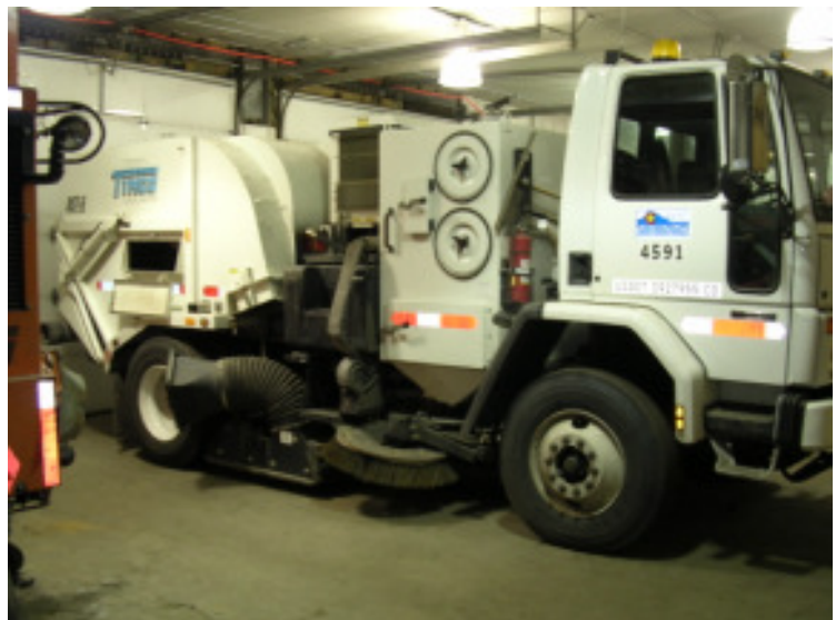
A vacuum sweeper used to remove sand and salt and meet PM 10 (air quality) requirements. The Denver metro area has four vacuum sweepers.
