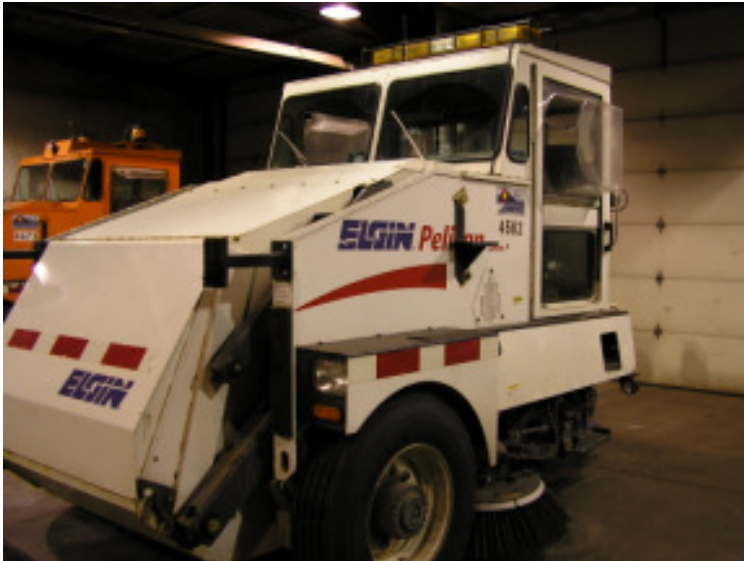
A regular broom used to remove sand and salt and meet PM 10 (air quality) requirements. With this sweeper, the material is swept up and later discarded. The Denver metro area has 12 regular brooms.
