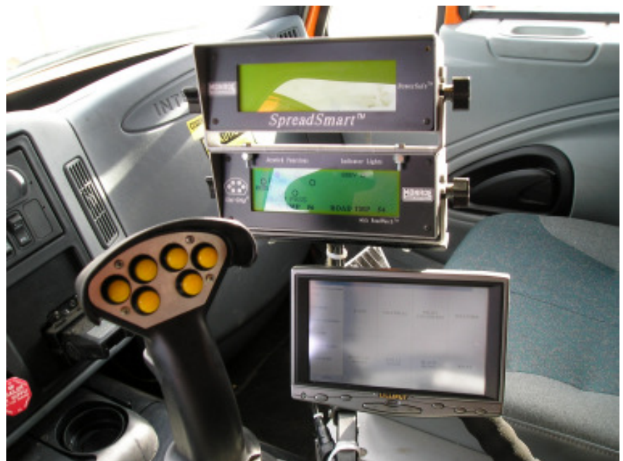
Five CDOT plow trucks in the metro area are equipped with a MDSS touch screen, which allows them to input real-time road and weather information.
