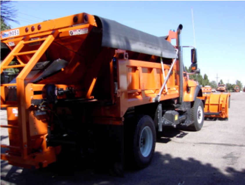
A mid-range plow with a V-box for applying solid de-icers. CDOT has 68 mid-range plows in the Denver metro area. Some of the mid-range plows are equipped with 1,000-gallon tanks for applying liquid de-icers and others are equipped to apply both solid and liquid de-icers.
