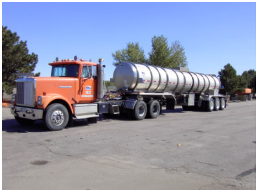
A 6000-gallon tanker used on I-25, I-70, US 36, US 6 and C-470 to spray liquid de-icers. The Denver metro area has three of these tankers.
