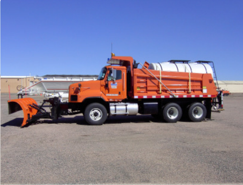
A tandem plow with a 1600-gallon liquid tank for applying liquid de-icers. CDOT has 36 tandems in the metro area, some have V-boxes for applying solid de-icers and some are combination trucks that can apply both solid and liquid de-icers.
